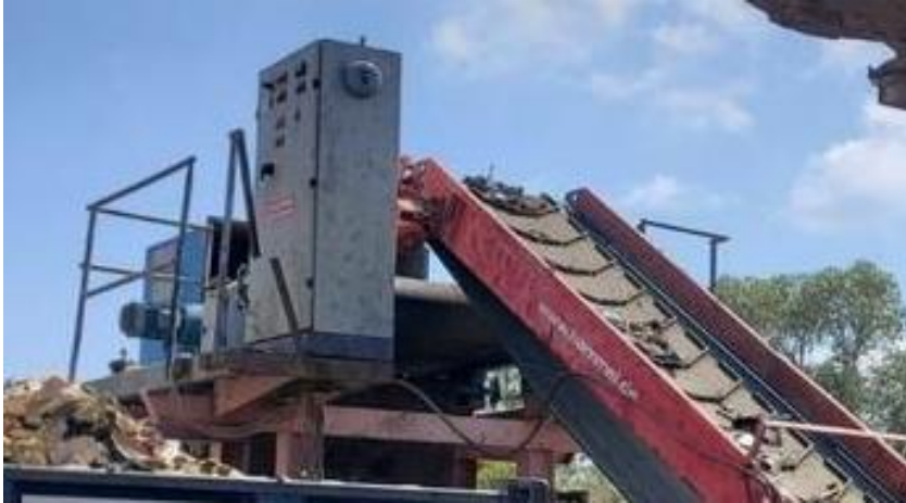
Figure 8: photographs of the installed equipment Model number for this is SGM Magnetics S.p.A. EIS100/150
